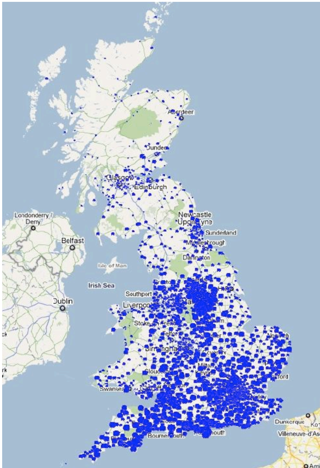
Figure 3: Density distribution Feed-in Tariff registered solar photovoltaic generation in the United Kingdom at 31 March 2011. Each blue circle represents the installed capacity in one postcode area at the resolution available to us, namely the leftwards portion (e.g. WC2N), and is located in the approximate centre of that area. The area of the blue circles is proportional to the installed capacity in that postcode area. Source: REF charting, from Ofgem data.
