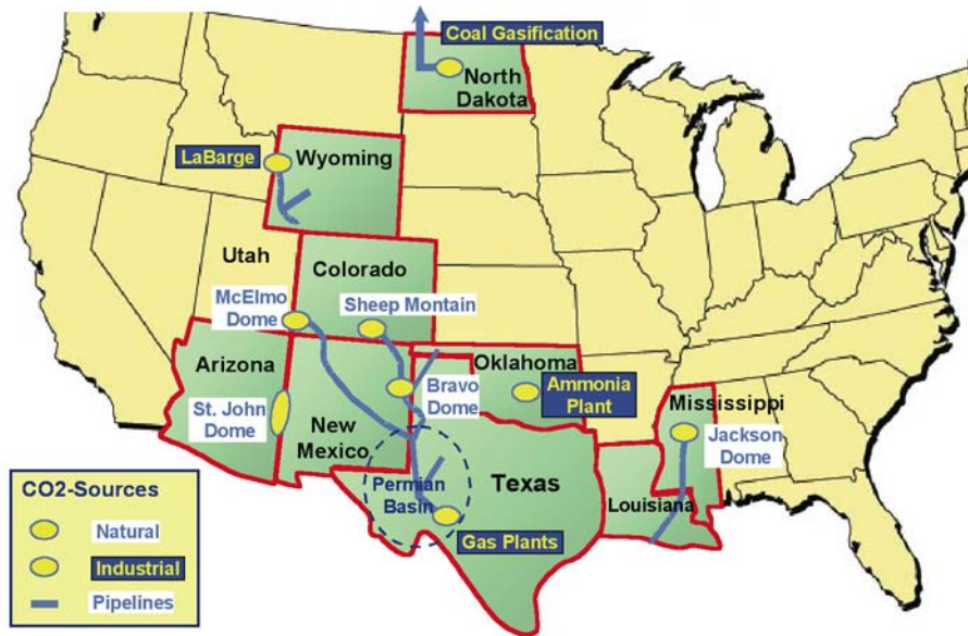
26. Network serving CO 2 for Enhanced Oil Recovery in the Permian Basin. Source: Kinder Morgan CO 2 Company.
